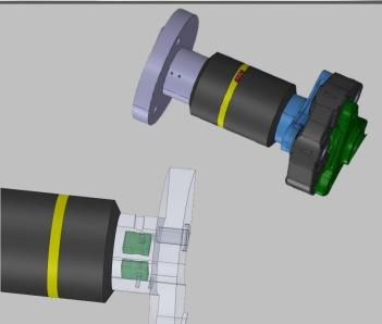
The J4T telemetry system allows simultaneous transmission of four thermocouple signals from rotating shafts. This installation provides four thermocouple female connectors for easy connection of the transducers. Sensor wiring comes through a hollow shaft from the differential gearbox.
