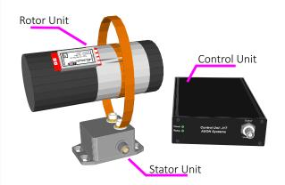
he telemetry system AXON J1T is designed for transmitting thermocouple based measurement signals from rotating shafts or other mechanical parts. Like all AXON telemetry systems, the J1T is extremely robust and delivers reliable readings at operating temperatures of up to +140°C in continuous operation, even under the toughest conditions. The inductive, contact-free power supply of Rotor Unit and transducer ensures an interruption-free operation.
