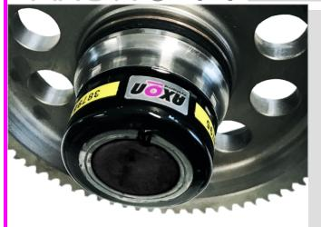
The highly effective inductive power supply of the rotating components allows an uninterrupted use even under harsh conditions.
