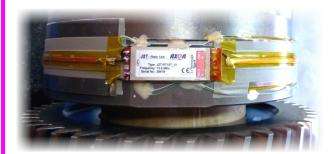
The highly effective inductive power supply of the rotating components allows an uninterrupted use even under harsh conditions.
