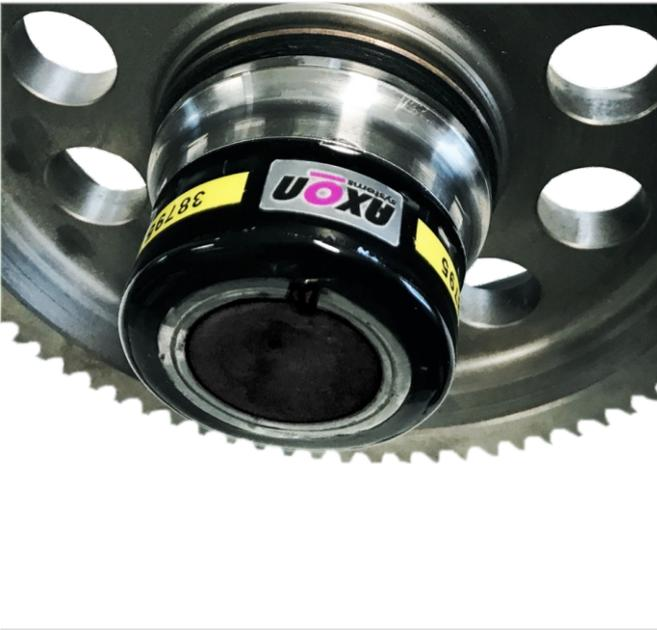
The highly effective inductive power supply of the rotating components allows an uninterrupted use even under harsh conditions.
