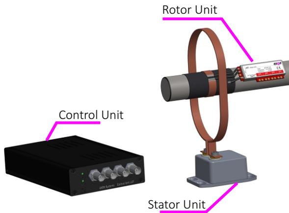
The telemetry system AXON J4T is designed for transmitting thermocouple based measurement signals from rotating shafts or other mechanical parts. Four sensors can be transmitted simultaneously. It combines smallest possible design with extreme robustness and delivers reliable readings at operating temperatures of up to +140°C in continuous operation, even under the toughest conditions. The inductive, contact-free power supply of Rotor Unit and transducer ensures an interruption-free operation.
