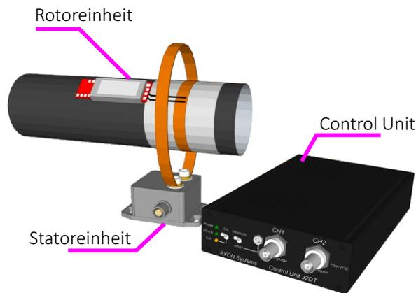
The telemetry system AXON J2DT transmits the signals of one strain gauge and one thermocouple at the same time. The amplified signals are made available on the Control Unit for further recording. The quality of the received digital data stream is constantly monitored, regulated and displayed via RSSI output. Thus, the telemetry system offers the possibility to simultaneously measure two sensor signals in the smallest space and transmit them contactless.
